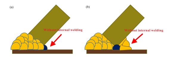
Fig.1. Two different welding designs of nodes: (a) in Europe and (b) in Taiwan. The blue area is the first bead.
