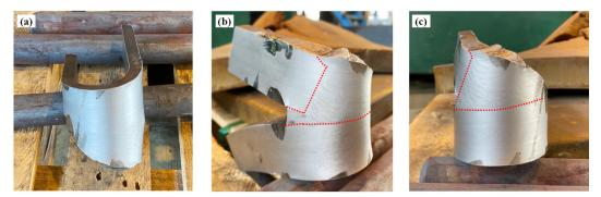
Fig.11. Results of the bending tests for node welding zone. The area indicated by the red dotted line is the weld bead.
