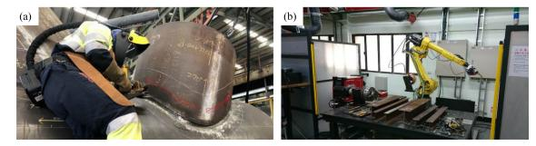
Fig.3. (a) Welding was manually performed in the shop, and (b) welding was done by a robot in the laboratory.
