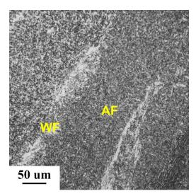
Fig.9. Microstructure of weld metal by FCAW.
