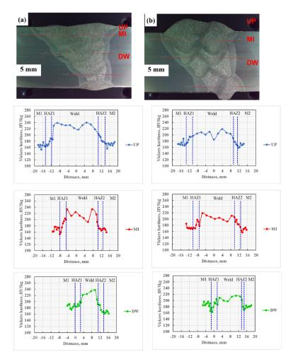
Fig.13. The macro-metallography of weldment and hardness distribution of (a) FCAW and (b) MCAW weldment
