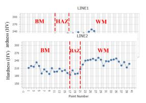
**Fig.10.** Hardness distribution of welding cross-section of a node.
